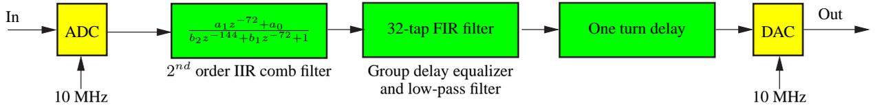
Figure 5: A block diagram of one channel of PEP-II double-peaked comb filter
