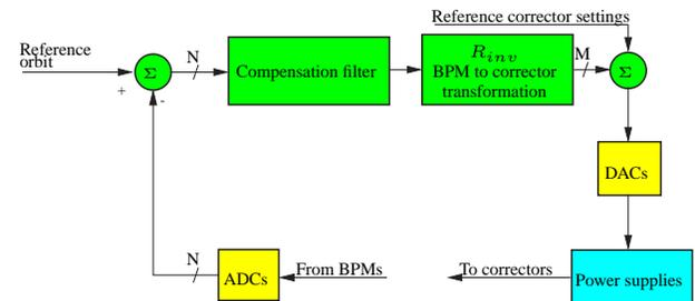
Figure 6: Block diagram of a global orbit feedback system
