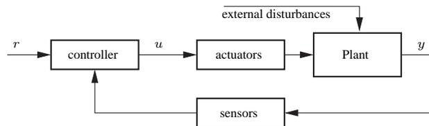
Figure 1: Generalized block diagram of a feedback system
