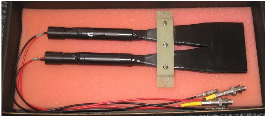
Figure 2.6: Trigger counter of single detector package.
