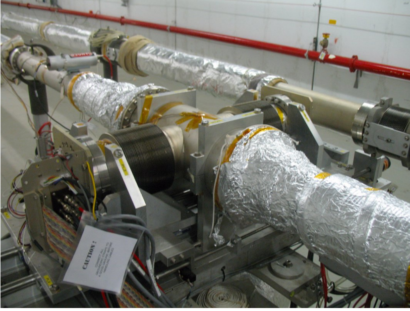
Figure 2.2: Horizontal station of Roman Pot detectors.
