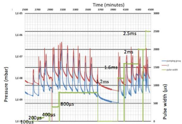
Figure 7: Pressure evolution during RF power cycles.
