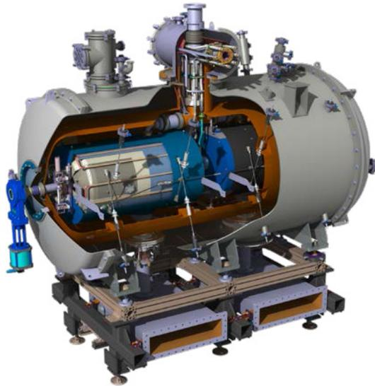
Figure 2. View of spoke cavity cryomodule.
