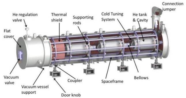
Figure 5: View of the ESS elliptical cryomodule.
