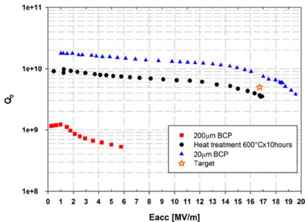
Figure 6: Q curves of the cavity MBP01.
