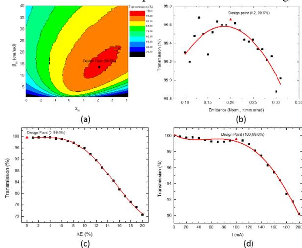
Figure 4: Transmission versus input twiss parameters (a), input beam emittance (b), input beam energy spread (c) and input beam current (d).
