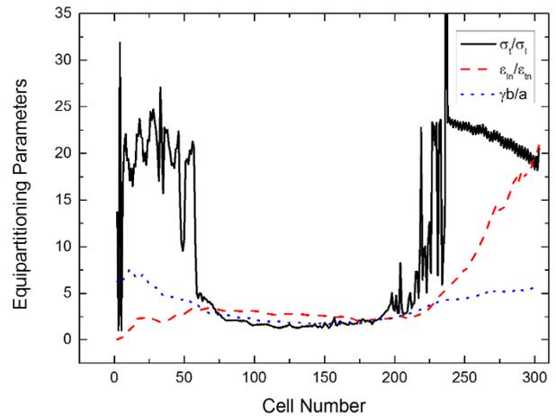
Figure 1: Equipartitioning parameters of this RFQ.
