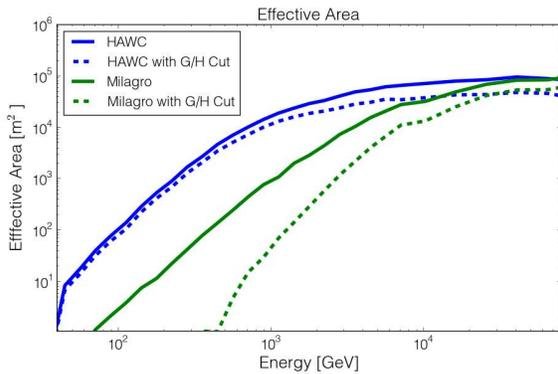
Figure 1: Effective area of HAWC along with the effective area of the predecessor experiment Milagro for comparison. Above about 1 TeV, the effective area approaches the geometrical footprint of the experiment and at lower energies the effective area is reduced due to the tendency of lower energy air showers to result in few energetic particles on the ground
