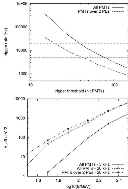
Figure 4: The top panel shows the trigger threshold required to obtain given threshold for different potential trigger algorithms. The bottom panel shows the effective area at trigger level for different potential trigger algorithms at 20 kHz rate along with the baseline. The potential for improvement at 100 GeV is evident.
