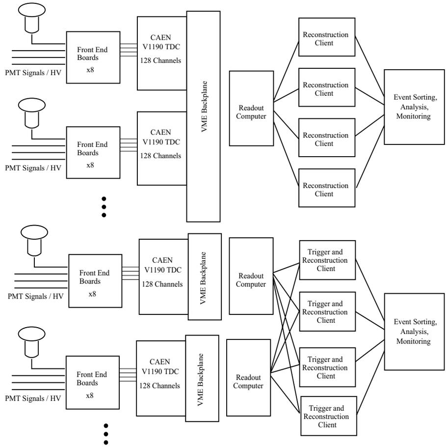
Figure 3: Two potential designs for the HAWC data acquisition system described in the text. The top figure is the baseline design and has all data read out across one VME backplane whereas the potential improvement in the lower figure does not have the same bottleneck.
