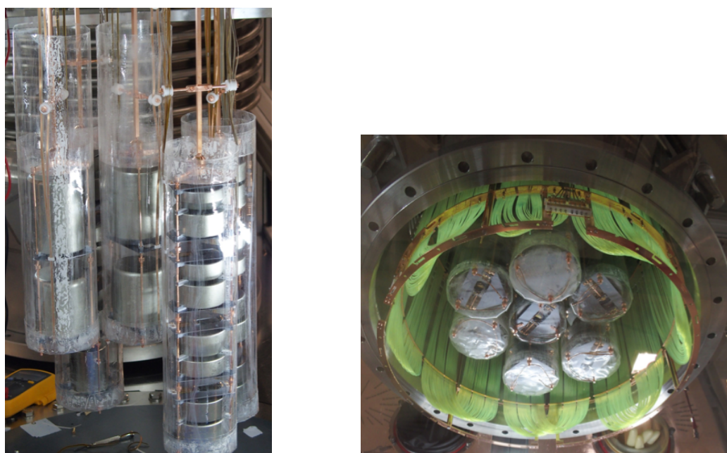
Figure 2. The Phase II Ge array with the individual Ge detector strings inserted in TPB coated nylon mini-shrouds (left) and the Fiber Shroud surrounding the detector strings once lifted up in the lock (right).
