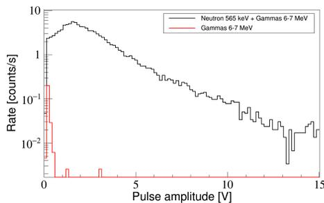
Figure 3: Response of the slow detector to the mixed field of 565 keV neutrons and 6-7 MeV gammas (black) and in the case of only gammas (red).
