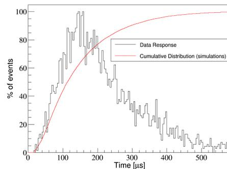
Figure 6: Time response for the slow detector as measured at IPHI following the 90  $\mu\text{s}$  proton beam pulse (black). The response is delayed with respect to the one obtained with the fast module due to the moderation process of the neutrons in the polyethylene. In red the cumulative distribution obtained from MonteCarlo simulations is also shown for an instantaneous pulse.
