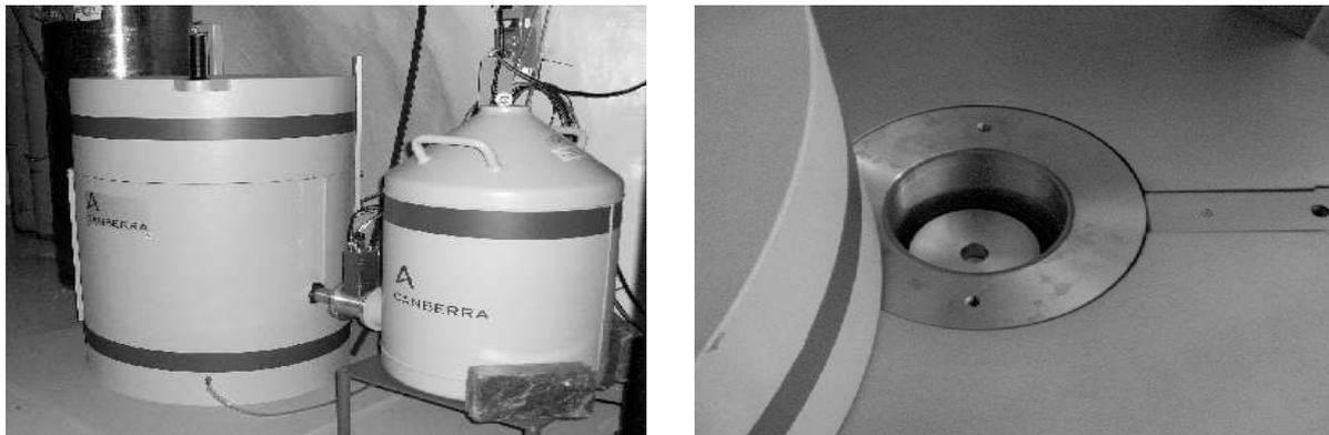
**Figure 3.** The SNOLAB Canberra germanium well counter. The right hand photo shows the detector and sample chamber.
