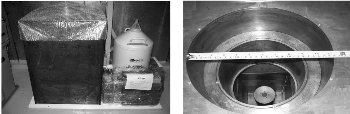
**Figure 1.** The SNOLAB PGT germanium counter, the copper box is used to prevent the ingress of radon into the detector chamber. The right hand photo shows the detector and sample chamber.
