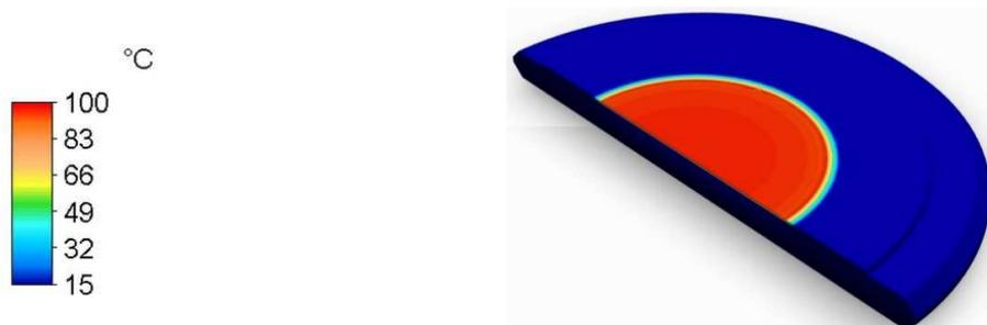
Figure 28: Temperature distribution of an assembly of thin disk and heat sink computed for no laser operation (fluorescence mode). The parameters of the thin disk parameters are given in the main text and in Table 4. The thermal load is  $50 \text{ W/mm}^3$  in the pumped active region.
