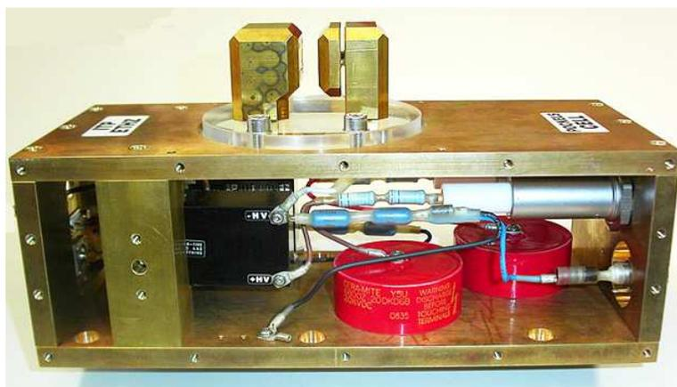
Figure 83: Picture of the Pockels cell without lateral walls and protective cap for the optical region. The optical region (top) is separated by an acrylic glass from the region containing the electronics (switches, capacitors etc.). 3D wiring minimizes the breakdown issues.
