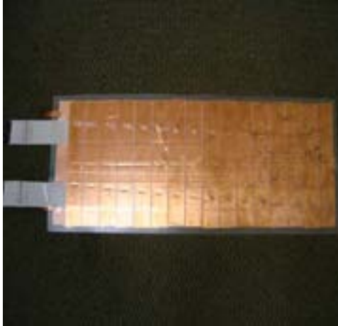
Figure 4, 5, 6: Z-plane before cloth was put on; Z-plane covered in cloth and taped to make it air tight; Z-plane after the thermal vacuum lamination process
