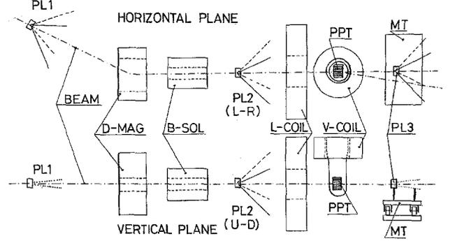
**Fig. 2.** The horizontal and vertical views of the proton beam line (not to scale). PL1, PL2 and PL3 are polarimeters, D-MAG is a bending dipole, B-SOL is the beam solenoid, L-COIL is the longitudinal holding coil, V-COIL is the vertical one. PPT is the polarized target and MT is the movable table
