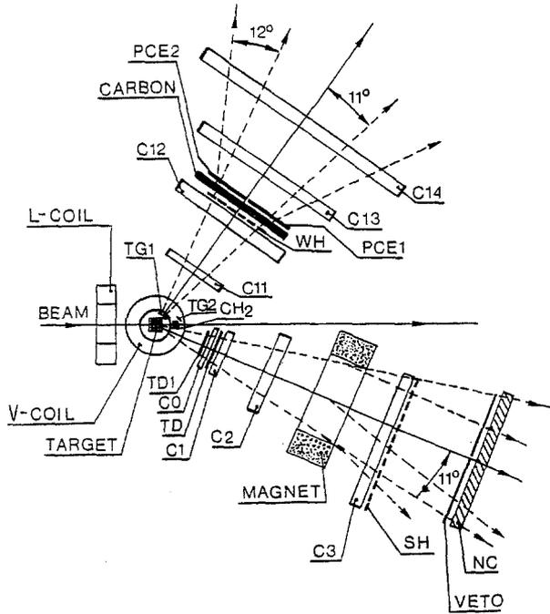
**Fig. 5.** The experimental set-up (not to scale). TD1, TD, TG1, TG2, PCE1, PCE2 were the single scintillation counters, SH, WH, “VETO” and NC were the counter hodoscopes, CARBON was the analyzer,  $CH_2$  was a small target, C0, C1, C2, C3, C11, C12, C13 and C14 were MWPC’s. Other symbols are as in Fig. 2
