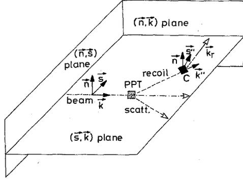
**Fig. 1.** The unit vectors  $\vec{n}$ ,  $\vec{s}$  and  $\vec{k}$  for the beam and target laboratory frame,  $\vec{n}$ ,  $\vec{s}$  and  $\vec{k}$  for the recoil particle frame and the  $\vec{k}_r$  is the rescattered recoil particle direction
