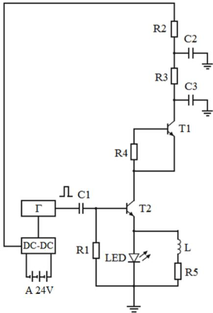
Figure 6: A system to calibrate the TUNKA-133 array from balloon or pilotless helicopter.
