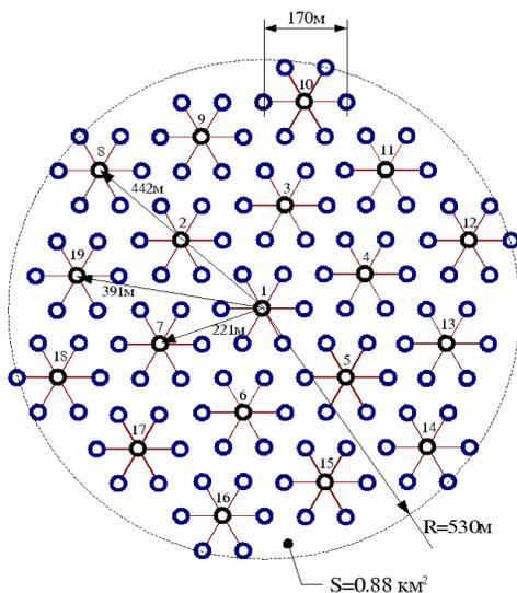
Figure 1. Layout of the TUNKA-133 EAS Cherenkov Array.
