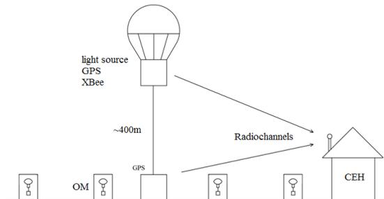
Figure 5: The concept of calibration of the TUNKA-133 array using light source attached to a helium balloon or a pilotless helicopter. Here OM is optical detectors and CEH is the central electronics hut of the array.
