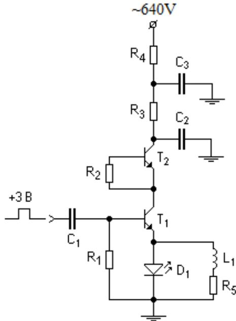
Figure 2: Electrical scheme of the light source.
