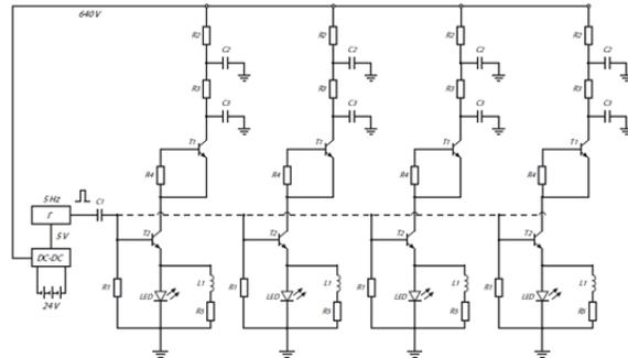
Figure 8: Electrical scheme of a system to calibrate the TUNKA-133 array using a complex light source raised above the TUNKA-133 array at the height of 2-3 m on a pole.
