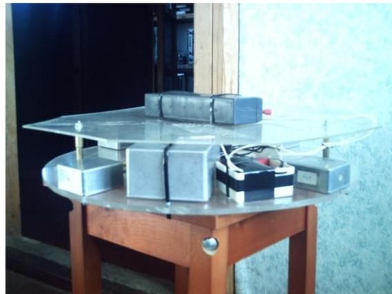
Figure 9: Photograph of the complex light source for calibration of the TUNKA-133 array using the light source hoisted on a pole at the height of 2-3 meters above the array.
