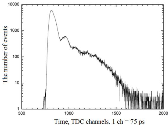
Figure 3: Light emission kinetics of the light source based on XR7090 high power LED.
