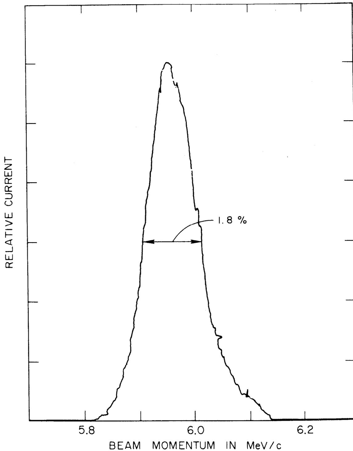
FIG. 5 TEST INJECTOR MOMENTUM SPECTRUM
