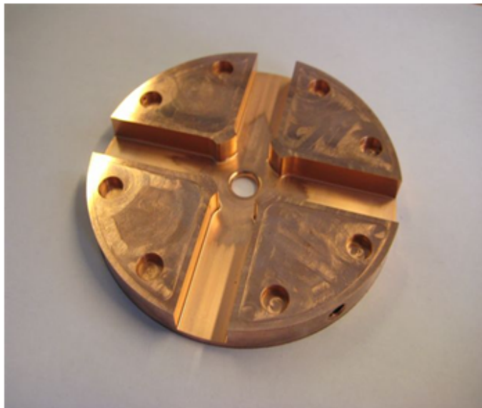
Figure 2.1: AS consists of copper disks, which are bonded together at near copper melting point.
