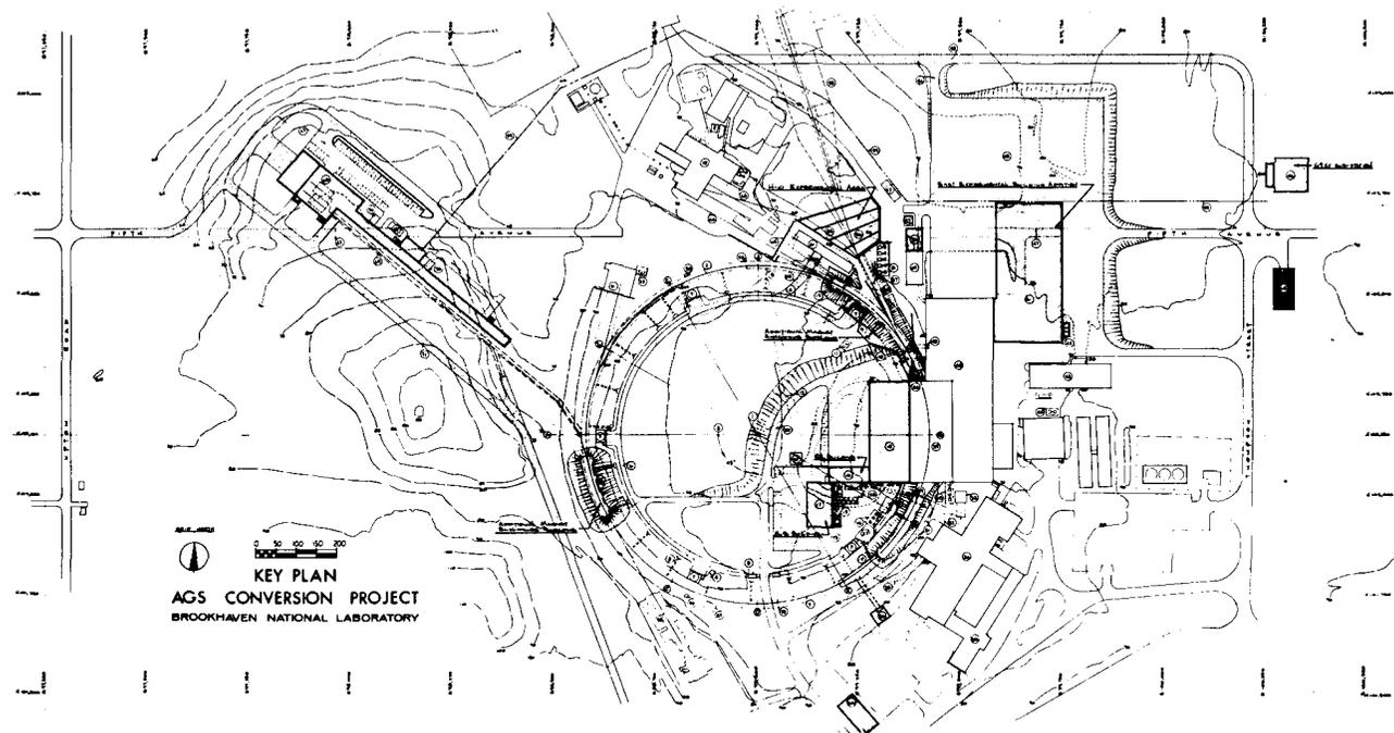
Fig. 5. Plot plan for the AGS Conversion Project.
