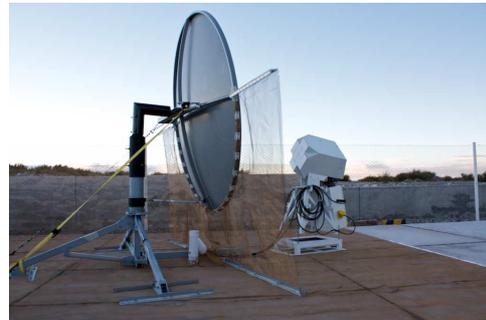
Figure 1: The upgraded AMBER antenna array installed at the HEAT enclosure at the Pierre Auger Observatory.
