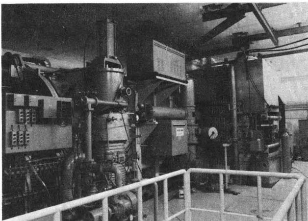
Fig. 2. The RCNP Isochronous Cyclotron. Main magnet, RF power amp, and RF resonator are seen at the right side, center, and left side of the photograph.
