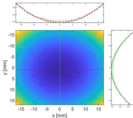
Figure 5: A slice of the longitudinal field inside the magnet's coil.
