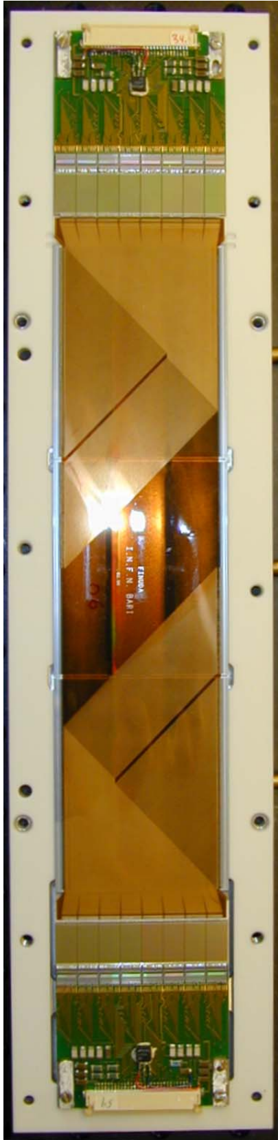
Figure 2.11: View of a module of the silicon vertex detector. The sensitive part is represented by three double sided silicon microstrip detectors glued head-to-head. At the extremities appear two hybrids each populated by 8 VA1 chips, which are followed by 8 charge-decoupling capacitors (larger chips).
