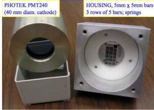
Figure 3. The housing made for the PHOTEK PMT240 (left) with three rows of angled bars. The quartz bars are held in a “crate” made by electro-erosion machining, such that the bars are only touched at their corners. Springs at the far ends of the bars apply a small pressure on the PMT240 window. Optical grease is used.
