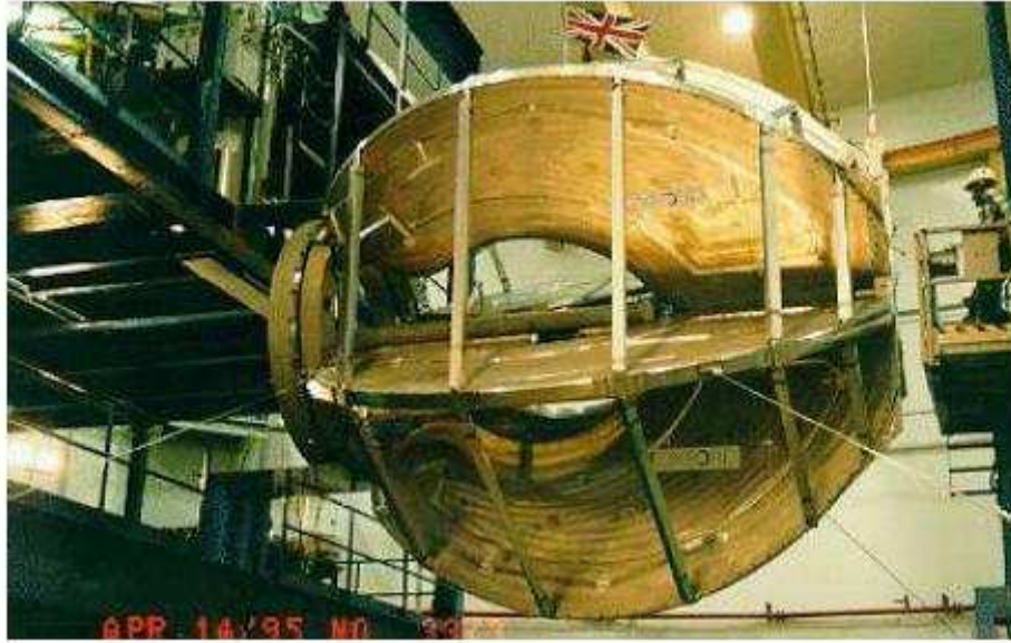
Figure 2.6: Photo of the CLAS Torus coils prior to installation. Image Source: [63]
