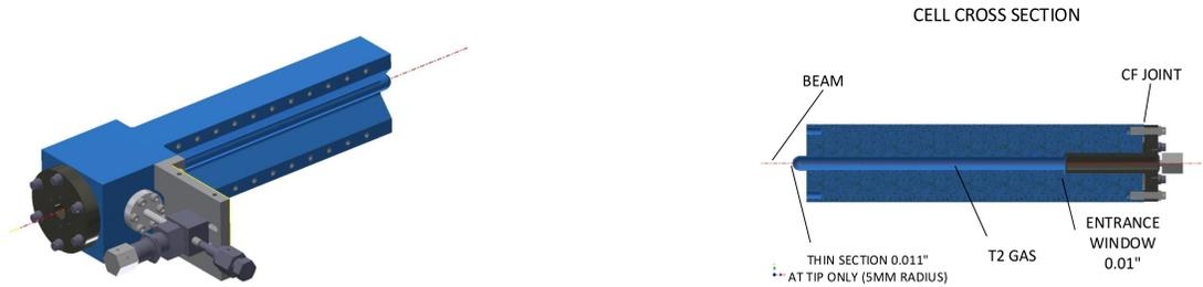
Figure 3.11: Tritium target cell design
