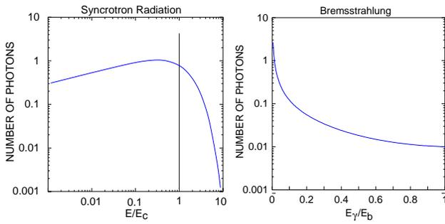
FIG. 4: Photon spectrum from synchrotron radiation and bremsstrahlung.
