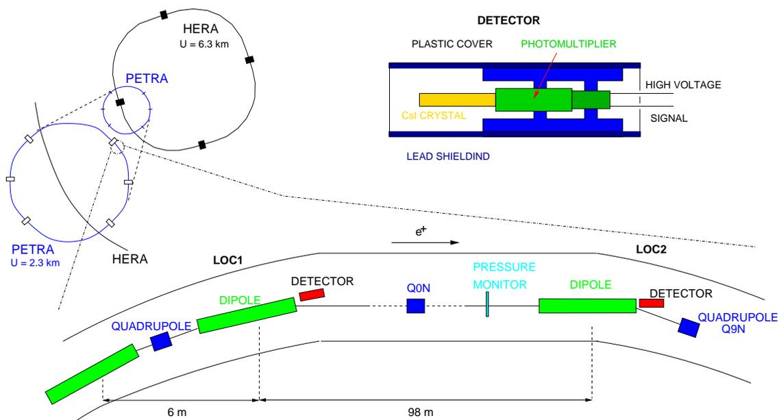
FIG. 8: Schematic setup for background measurements at PETRA.
