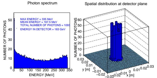
FIG. 5: Photon spectrum of Compton photons simulated with Geant4. Scattering of a 10 MW peak power green ( $\lambda = 532$  nm) laser beam with 1  $\mu\text{m}$  spot size at a 4.5 GeV electron beam with transverse beam size of 100  $\mu\text{m}$ . For the spatial distribution calculation the detector place was set 4 m away from the interaction.
