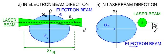
FIG. 1: Scheme of a gaussian laser beam focused to its diffraction limit scanned over an electron beam.
