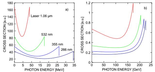
FIG. 3: Compton cross section for the first four harmonics of an Nd:YAG laser scanning a 1 GeV (a) and 250 GeV (b) electron beam.
