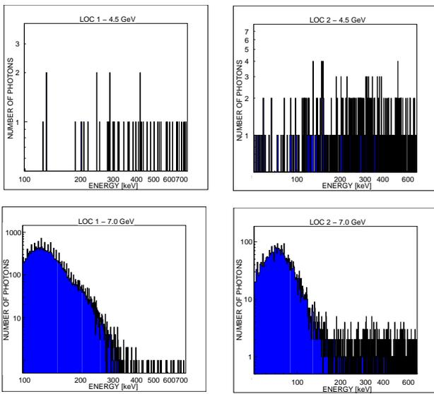
FIG. 6: Background spectra measured at PETRA. Data was taken over a 1 sec long period for each measurement.
