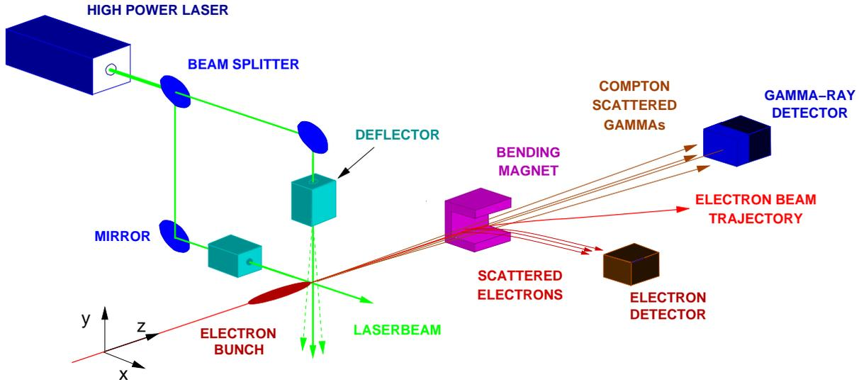
FIG. 7: Schematic setup for a laser wire beam profile monitor.
