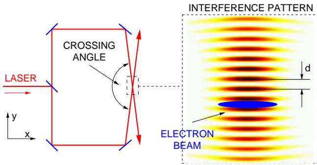
FIG. 2: Scheme for the generation of an interference pattern with fringe spacing  $d$ .
