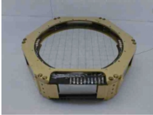
Figure 4.1: A photograph of the phonon sensor side of a mounted FLIP detector. Note the gold plated copper housing, the angled posts, Kapton copper circuit board, and the row of ten millmax sockets.
