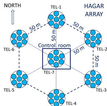
Figure 1: Schematic layout of HAGAR array
