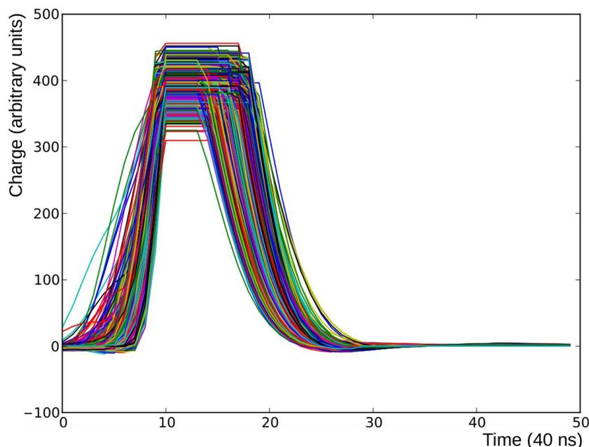
**Figure 8.11:** A selection of saturated waveforms in data, showing the saturation plateau. Plot provided by Lukas Koch.
