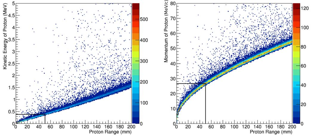
**Figure 2.6:** Plots the predicted range of protons in the drift gas of the ND280 TPCs as a function of kinetic energy (left) and momentum (right), from particle gun simulation. Limits are drawn on to show the anticipated minimum track length for successful reconstruction, showing that in this medium there is the potential to reconstruct protons with as little kinetic energy as 0.4 MeV.
