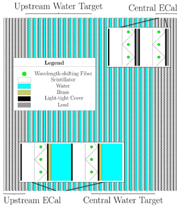
**Figure 3.9:** A diagram showing the construction of the P0D [3], with the beam entering from the left. The triangular segmentation of the scintillator bars is shown in close-up in the insets.
