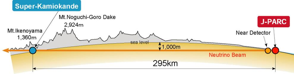
**Figure 3.1:** A diagram illustrating the layout of the T2K experiment [3]. Modified for clarity by T. Ishida.
