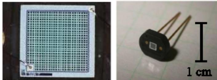
**Figure 3.10:** An MPPC of the type used in the ND280 P0D, FGDs and ECals. Left: magnified view of MPPC face, showing  $26 \times 26$  pixel array. Right: ceramic package of the same MPPC.
