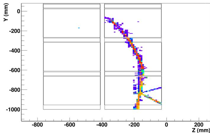
**Figure 8.9:** Y-Z view of the event shown in Figure 8.6, with a colour scale corresponding to the hit charge (in arbitrary units). No fitted tracks are drawn. A thin core of saturated (red and orange) MicroMEGAS hits can be observed following the “true” particle track; the surrounding blue hits have a very low charge. This is consistent with cross-talk from the saturated hits creating low-charge hits in neighbouring pads.
