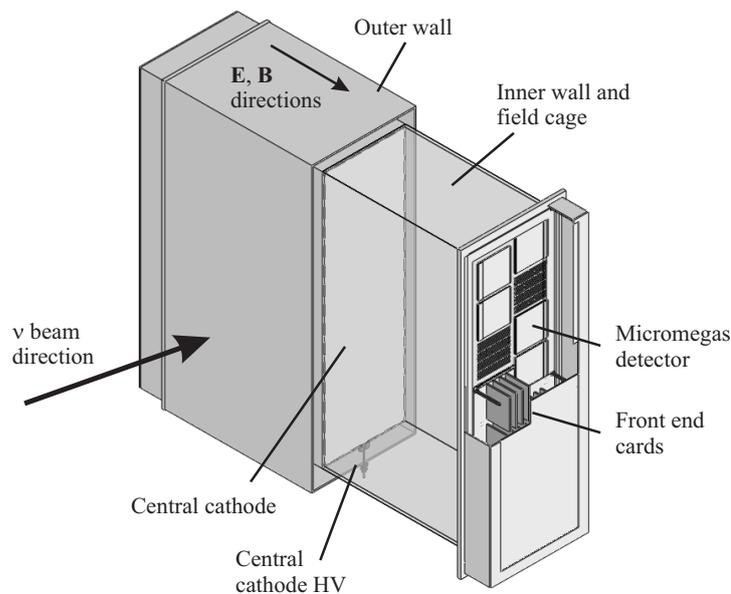
**Figure 3.12:** Cutaway drawing showing the TPC design [3]. The outer box has dimensions  $2.30 \times 2.40 \times 0.97$  m ( $x \times y \times z$ , where  $z$  is the beam axis and  $y$  is normal to the surface of the earth); the active gas volume contains 3,000 L of gas mixture, with a further 3,300 L in the gap volume between the field cage and the outer wall.
