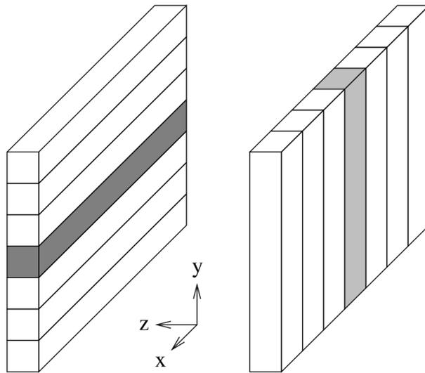
**Figure 3.11:** Illustration of the perpendicular layer configuration for the FGDs and ECals. The shaded bar on the left has its  $y$  coordinate defined by the bar and its  $z$  coordinate defined by its layer; the shaded bar on the right has its  $x$  coordinate defined by the bar and the  $z$  coordinate defined by its layer. Combining the 2D information from successive alternating layers allows for the reconstruction of a complete 3D track. Figure drawn by Luke Pickering.
