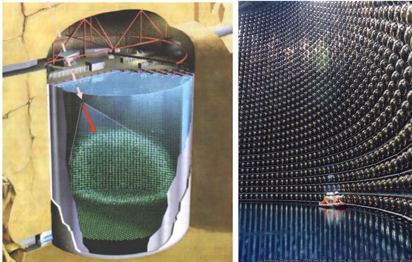
**Figure 3.14:** A diagram illustrating a neutrino interaction in Super-K from the Super-K website (left), and a photograph of the detector's interior wall (right).
