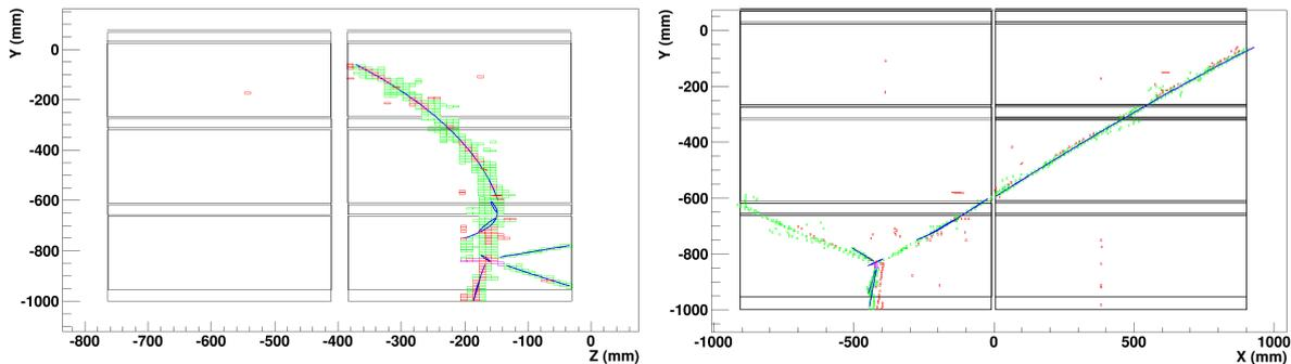
**Figure 8.6:** Orthogonal views of an event in the selected data sample with an unexpectedly thick, noisy track emerging from the vertex. Green boxes indicate MicroMEGAS hits used by the pathfinding, red boxes hits which were not used, and purple boxes hits that were assigned to a junction. Blue lines indicate fitted paths, and red lines paths for which the fitting failed. X is the drift axis and Z is the beam axis.
