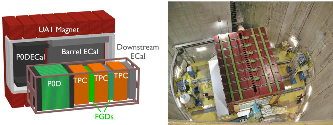
**Figure 3.8:** An exploded cross-section of ND280 [3] (left), and a photograph of ND280 with the magnet closed (right).
