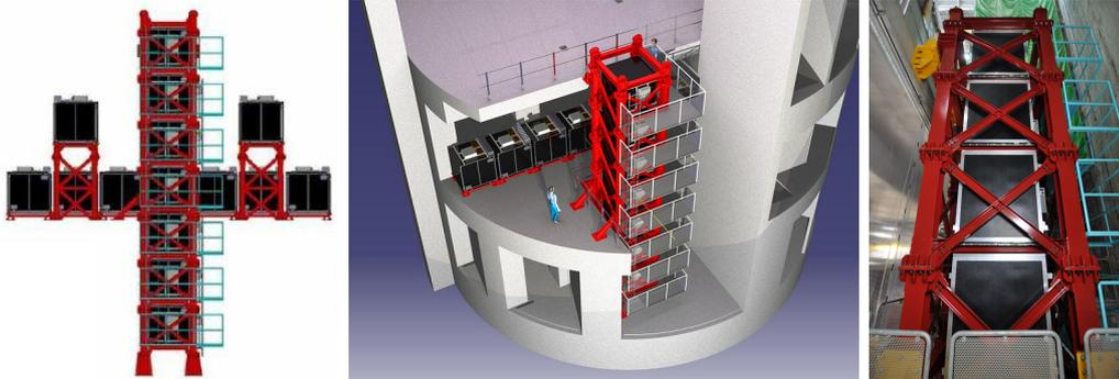
**Figure 3.6:** A diagram showing the layout of the INGRID detector as seen from the beam direction [3] (left), a diagram showing the placement of INGRID in the pit (centre), and a photograph of INGRID's vertical modules (right).
