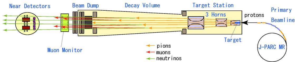
**Figure 3.5:** A schematic of the secondary neutrino beamline. Official T2K figure provided by T. Ishida.
