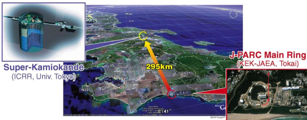
Figure 2.1: The neutrino beam journey in the T2K experiment. The high intensity neutrino beam is produced at J-PARC (Tokai, Mito, Ibaraki Prefecture, Japan) and travel 295 km to the Super-Kamiokande detector (mount Kamioka, close to Hida, Gifu Prefecture, Japan).
