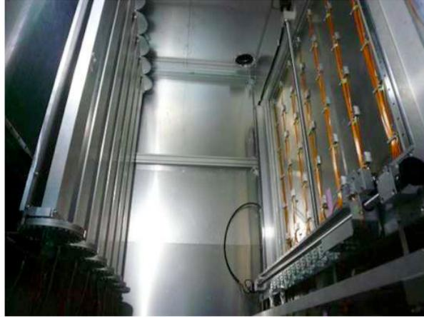
Figure 2.17: Muon monitor inside the support enclosure. The silicon PIN photodiode array is on the right side and the ionization chamber array is on the left side. The muon beam enters from the left side.
