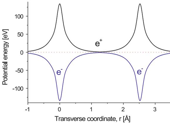
**Fig. 2** The transverse potential energy for positrons and electrons, in the continuum approximation, for diamond along the  $\langle 110 \rangle$  axis at room temperature. The main regions for channelled  $e^-$  and  $e^+$  are indicated. The Doyle-Turner approximation for the atomic potential has been used [1]
