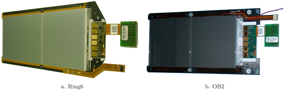
Figure 3.2: Modules of two different types. A wedge shape detector module for the Tracker Endcap of Ring6 geometry is shown in Fig. a and a module for the Outer Barrel in Fig. b.
