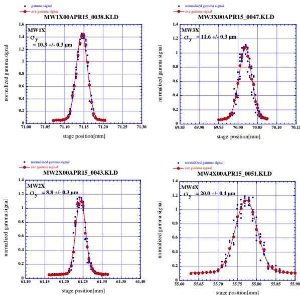
Figure 3: Vertical wire scans in the EXT, using W filaments with  $10\mu\text{m}$  diameter.
