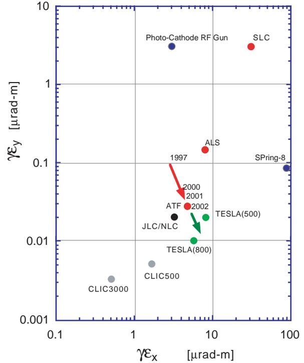
Figure 1: Comparison of the normalized emittance.
