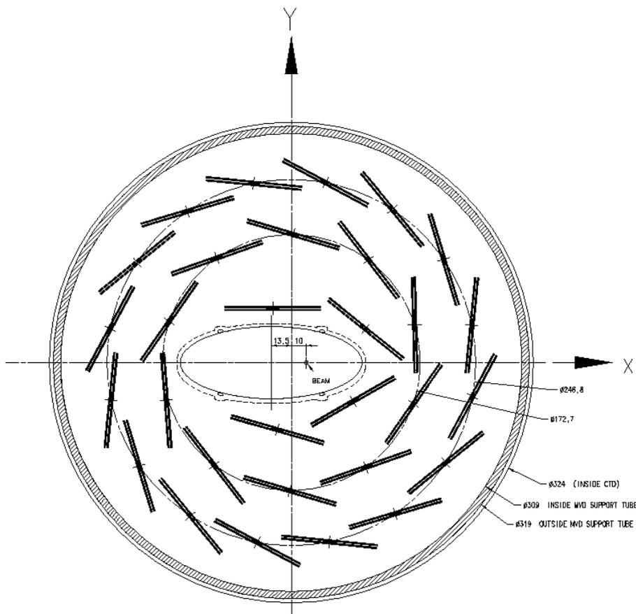
Figure 3.10: Cross section of the layout of the silicon sensors in the barrel MVD.
