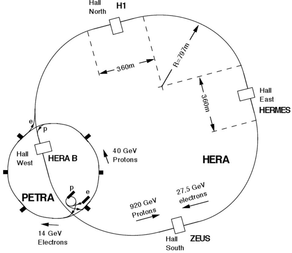
Figure 3.1: Scheme of the HERA collider ring.
