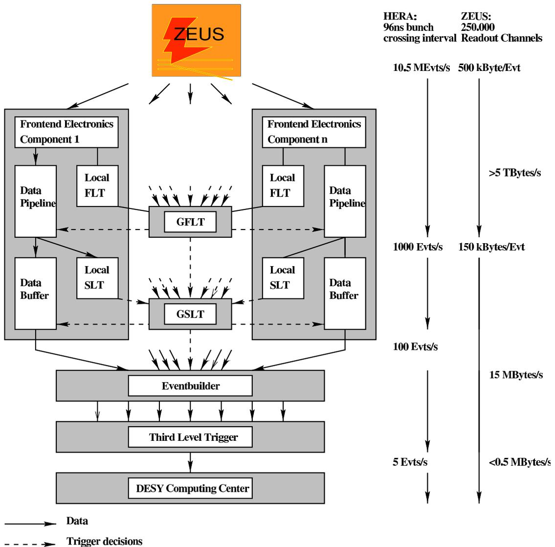
Figure 3.12: A scheme of the ZEUS trigger system [115].
