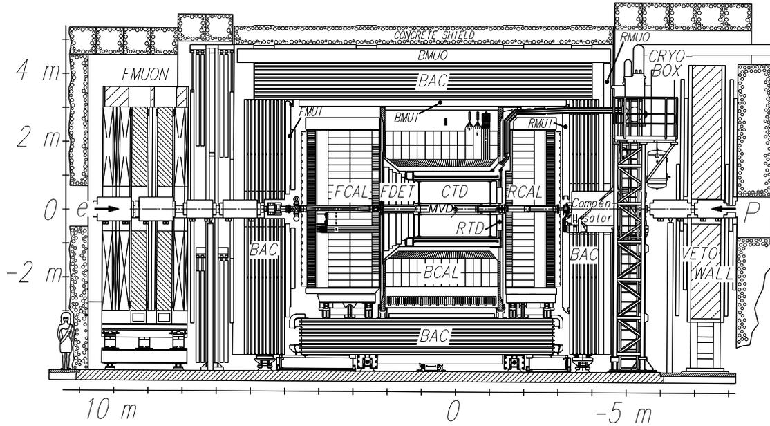
Figure 3.5: Side-view of the ZEUS detector.
