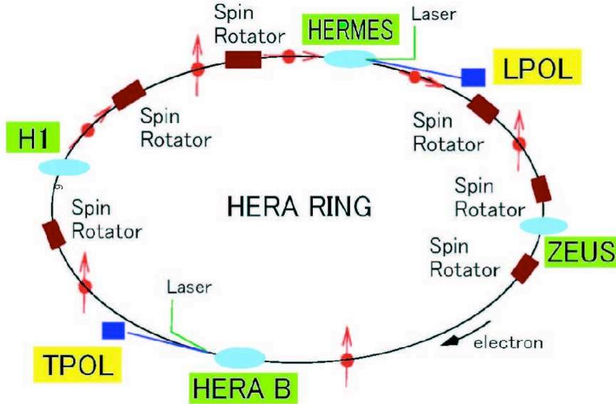
Figure 3.4: The locations of spin rotators and polarimeters around the HERA ring. The arrows represent the directions of leptons' spins at different points around the ring.
