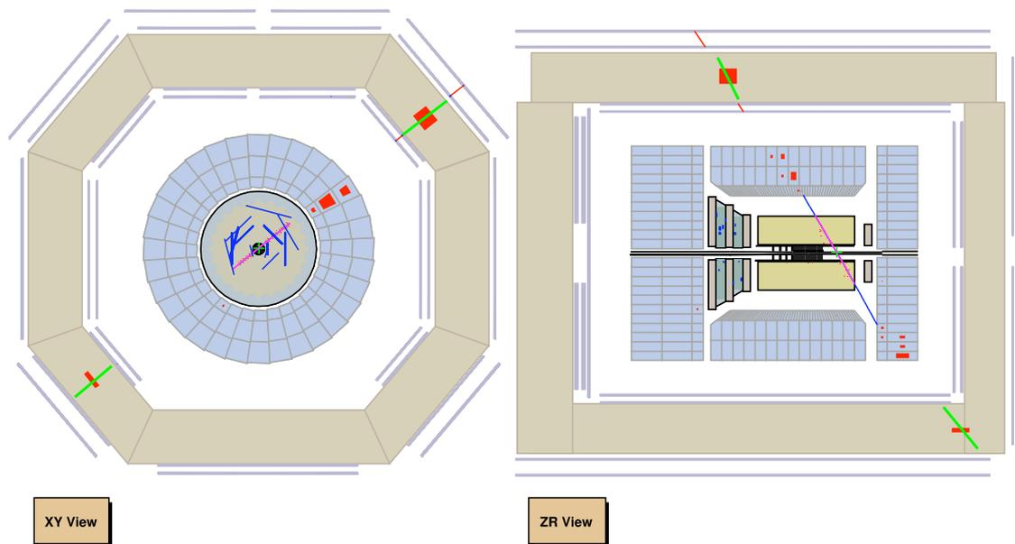
Figure 5.3: An example of a cosmic muon event.
