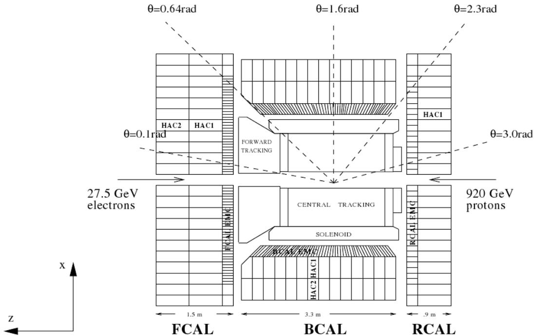
Figure 3.8: Side-view of the ZEUS calorimeter.
