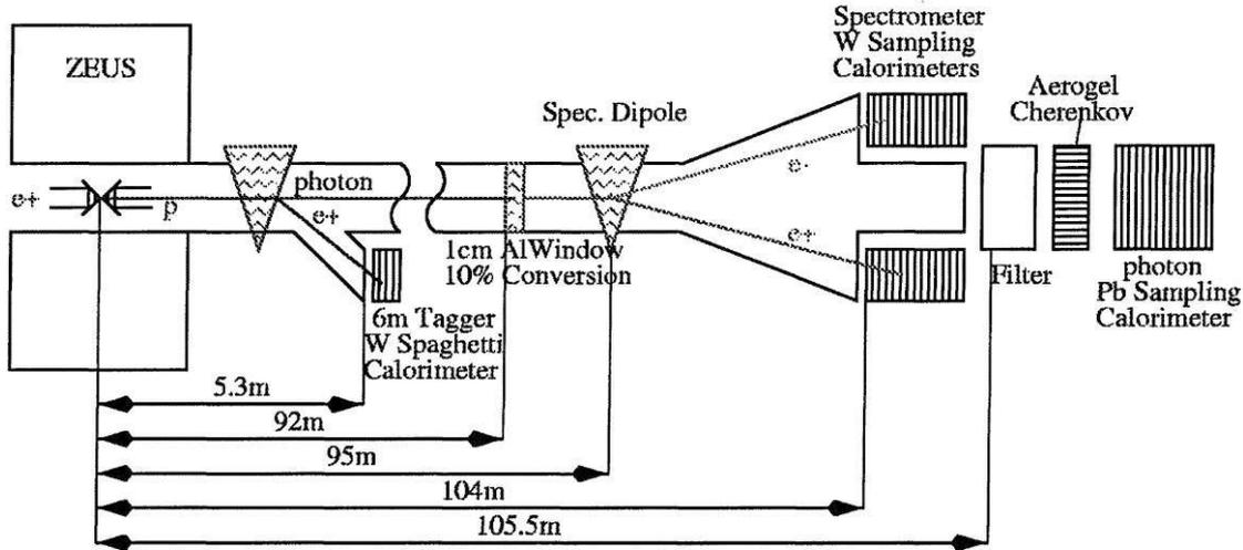
Figure 3.11: General layout of the ZEUS luminosity system.
