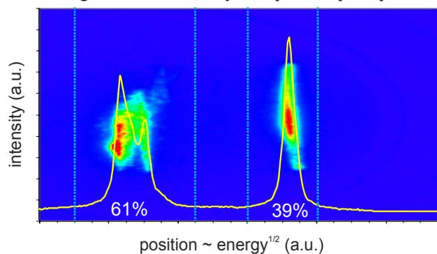
Figure 2: Energy spectrum of ions after the IH. The dashed lines indicate the areas used for integration. The rightmost peak corresponds to 0.5 MeV/u and the leftmost one to 4 MeV/u.
