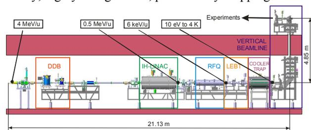
Figure 1: Overview of the HITRAP facility with the major components indicated. DDB: Double Drift Buncher for bunching the beam to adapt it to the longitudinal acceptance of the decelerator, IH-LINAC: Interdigital H-type structure for deceleration, RFQ: Radio-Frequency Quadrupole accelerator structure for deceleration, LEBT: Low-Energy Beam Transport line for efficient injection into the trap, COOLER TRAP: Penning trap for final deceleration and cooling.
