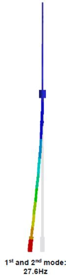
Figure 10.16: If it is assumed that the magnets are fixed and that there is sufficient clearance in the bearings then the lower part of the shaft will have a resonance at 27.6 Hz[120].
