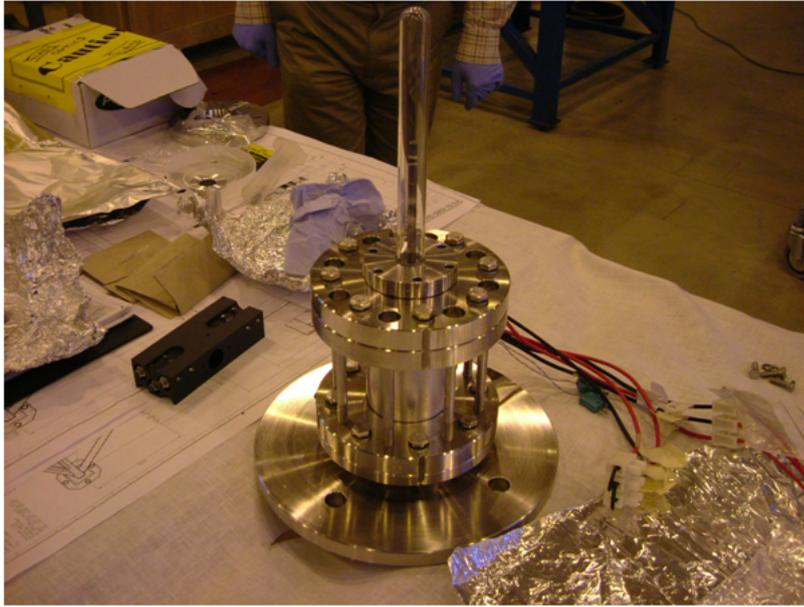
Figure 6.9: The glass tube on top of the stator can be seen in this photograph with a prototype optics block loaded with collimators on the left.
