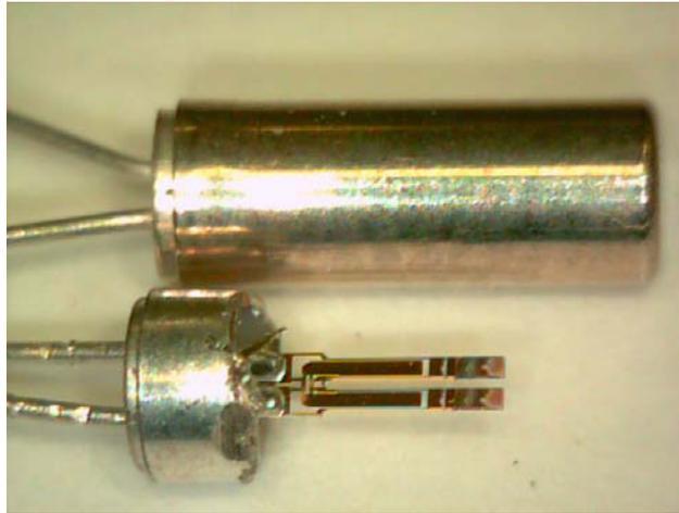
Figure 1. Quartz tuning fork, in capsule and with opened package
