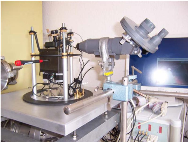
Figure 5. AFM with standard head and optical positioning aid
