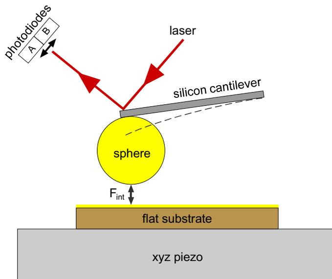
Figure 2. Basic principle of measuring force with a cantilever and bounced laser beam
