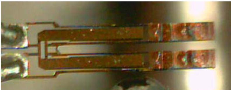
Figure 4. Quartz tuning fork and metal ball
