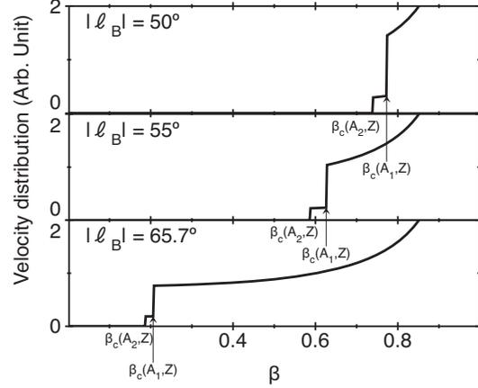
Figure 1: Velocity distribution of vertical incident  $Z = 4$  charged particle with atomic mass number  $A_1=9$  and  $A_2 = 10$  expected to be measured at (from top to bottom)  $50^\circ$ ,  $55^\circ$  and  $\sim 66^\circ$  of geomagnetic latitude.
