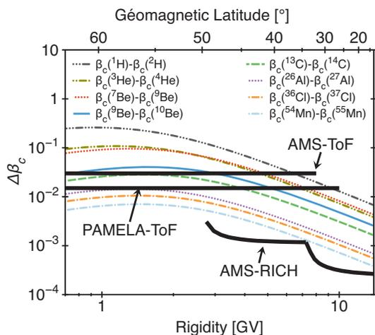
Figure 3: Differences  $\Delta\beta$  in threshold velocity for various couple of isotopes of interest in the study of the cosmic-ray diffusion. For comparison, the thick lines indicate the velocity resolution of the AMS-ToF, AMS-RICH (taken from [2, 3]) and PAMELA-ToF (taken from [4]).
