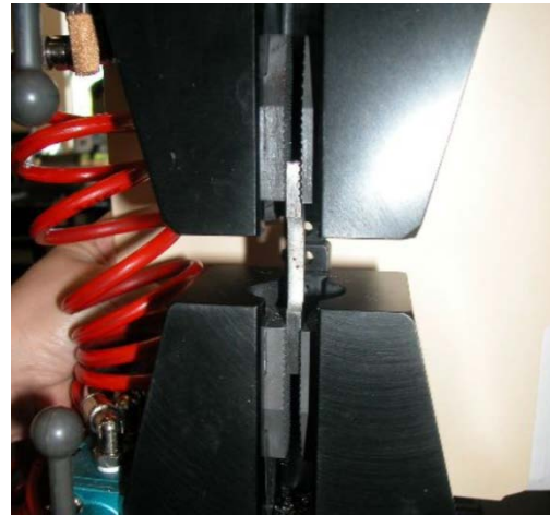
Figure 9 : Setup for a tensile test on a strip cut from one of the large sized specimens.
