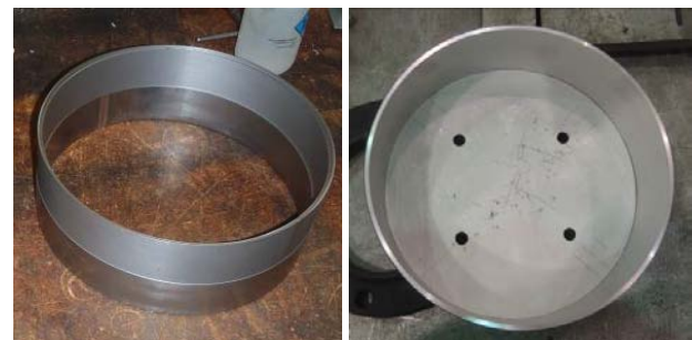
Figure 6 : The two large trial pieces. One without plug (left) and one with a 1 inch thick plug (right).
