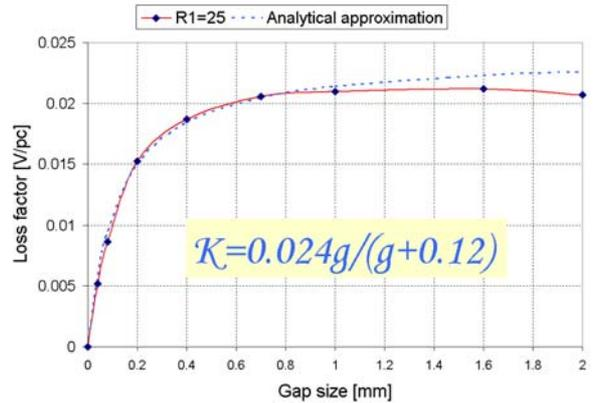
Figure 6: Comparison of the calculate values for loss factor  $K$  with the analytical approximation.
