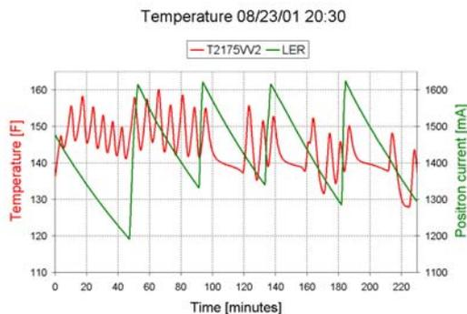
Figure 1: Vacuum valve temperature and positron current.
