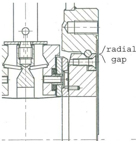
Figure 8: Vacuum valve flange geometry.
