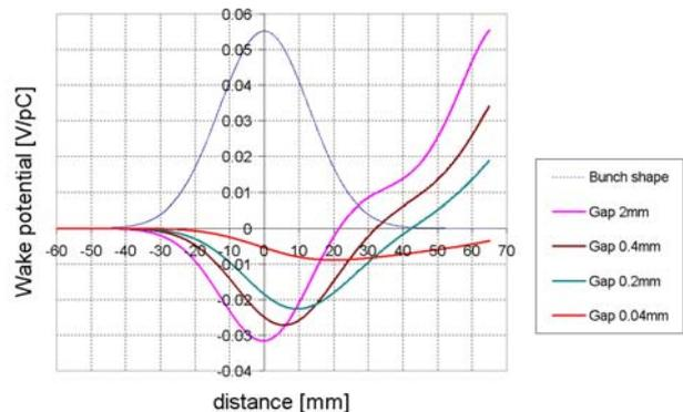
Figure 3: Wake potentials for a bunch length of 13mm for different gap sizes.
