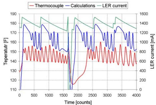
Figure 10: Comparison of the simulated temperature oscillations (blue middle curve) and measured temperatures from the thermocouple (red down curve) with the positron beam current (green upper curve) as a function of time.
