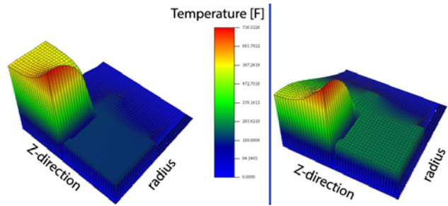
Figure 9: Temperature distribution in the vacuum valve flange connection for different stages of the thermal contact. Maximum temperature is achieved at the inner edge of the stainless steel vacuum valve flange.
