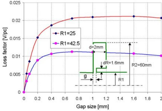
Figure 4: Loss factor as a function of the gap size.
