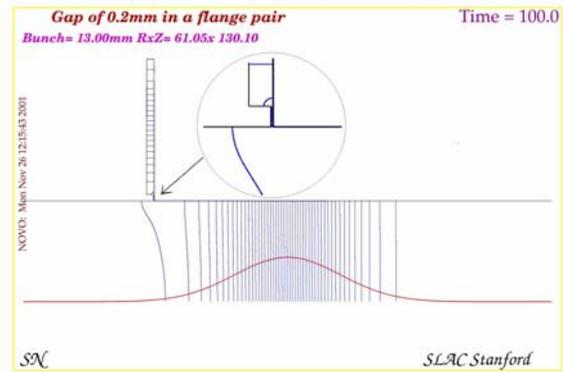
Figure 2: Electric force lines of the field excited by a bunch, travelling in the vacuum chamber with a small gap.
