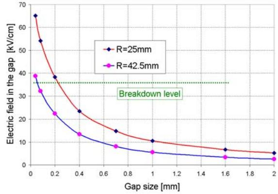
Figure 5: Amplitudes of the electric field in the gap for different gap sizes.
