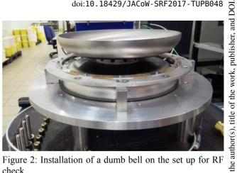
Figure 2: Installation of a dumb bell on the set up for RF check.
