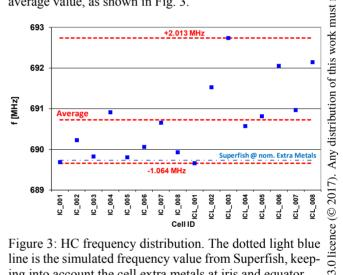
Figure 3: HC frequency distribution. The dotted light blue line is the simulated frequency value from Superfish, keeping into account the cell extra metals at iris and equator.
