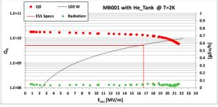
Figure 10: Performances of MB001 integrated in the He-Tank.
