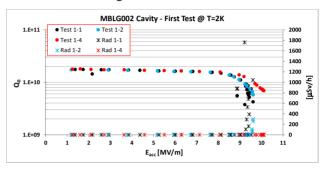
Figure 12: MBLG002 Q<sub>0</sub> vs E<sub>acc</sub> plots showing FE.
