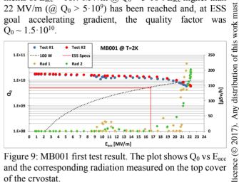
Figure 9: MB001 first test result. The plot shows Q<sub>0</sub> vs E<sub>acc</sub> and the corresponding radiation measured on the top cover of the cryostat.
