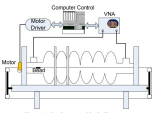
Figure 4: Tuning setup block diagram.
