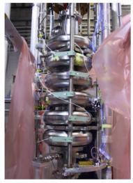
Figure 7: MB001 cavity installation on the insert.
