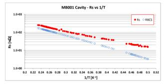
Figure 8: MB001 R<sub>s</sub> behaviour during sub-cooling from 4.2 K to 2 K.
