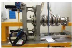
Figure 5: MB prototype cavity placed on the tuning machine.
