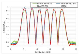
Figure 6: MB001 cavity field profile evolution before and after "Bulk BCP" and after final tuning.
