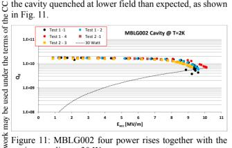
Figure 11: MBLG002 four power rises together with the equi-power line at 30 W.
