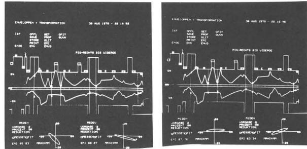
Fig. 6 Calculated envelopes on the basis of emittance measurements (+ measured profile width)
