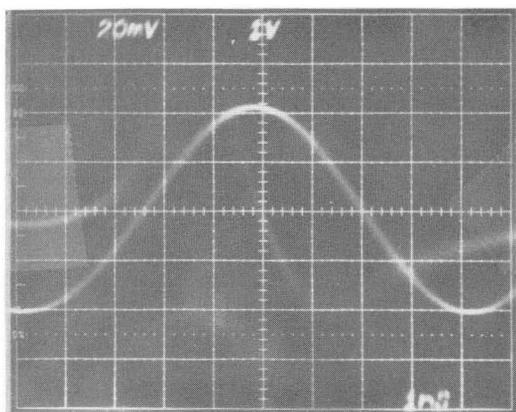
Fig. 2b Bunch position with respect to the rf signal of the first Alvarez cavity
