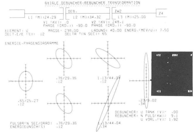
Fig. 4 Output of the program for the rebuncher-debuncher system (right: measured bunch width on the target)
