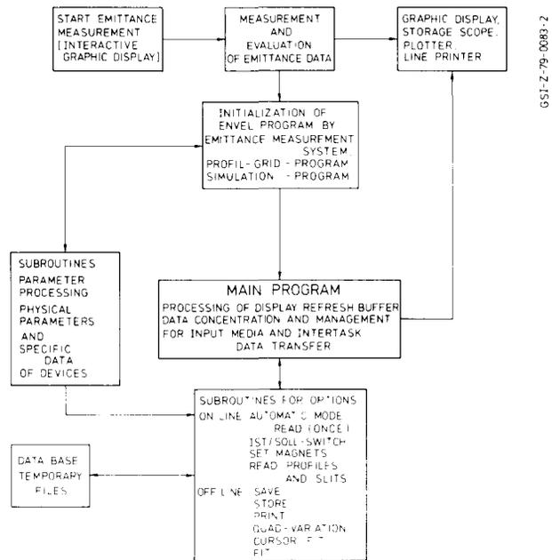
SCHEMATIC DIAGRAM OF THE PROGRAM STRUCTURE FOR TRANSVERSE BEAM OPTIMIZATION
