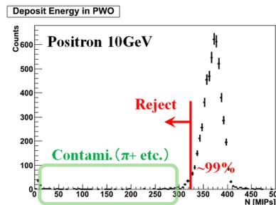
Figure 4: Quality cut of contamination particles by using energy deposit in TASC.
