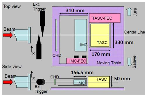
Figure 1: Detector setup of the beam test.
