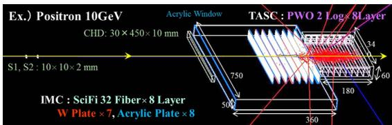
Figure 5: Overview of CALET prototype detector and shower of 10 GeV positron drawing by Geant4 simulation.
