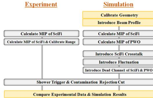
Figure 3: Comparison of data analysis procedure of experiment and simulation.
