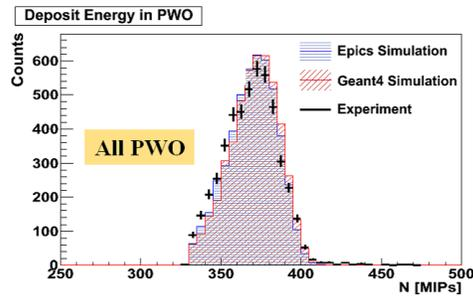
Figure 7: Experimental result of energy deposit in all PWO logs by 10 GeV e+, in comparison with Geant4 and EPICS.
