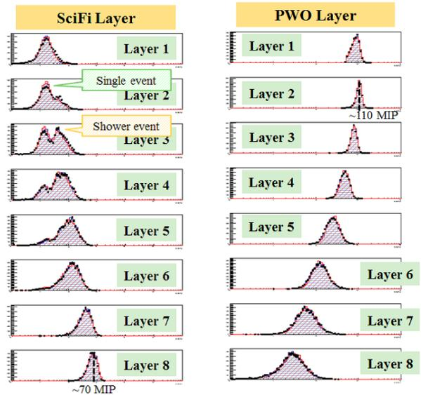
Figure 8: Energy deposit in each SciFi layer, in which the shower starting point is clearly seen.
