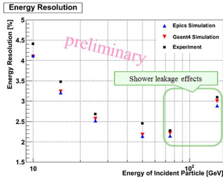
Figure 10: Energy resolution of TASC for positrons.
