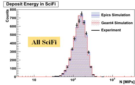
Figure 6: Experimental result of energy deposit in all SciFi's by 10 GeV e+, in comparison with Geant4 and EPICS.
