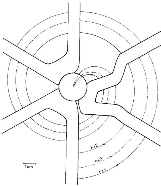
Fig.2 : Constant trajectories in the median plane corresponding to each harmonic mode, and shapes of the first accelerating gaps.
