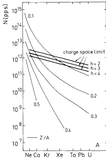
Fig.3 : EBIS-type of an ion source : inferior limits of the intensities  $N$  (p.p.s) at the cyclotron exit for electronic beam density of  $J_c = 10^4$  A/cm<sup>2</sup>. One supposes an overall 10% efficiency. The charge space limit related to a  $\pm 1.5^\circ$  bunching has been estimated within the frame of the "spherical bunch" model. (eq. 4,5,6).
