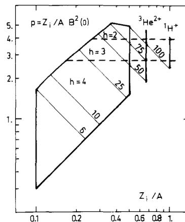
Fig.1 : Diagram of the possible values of  $p = \frac{Z_i}{A} B^2(0)$  and the regions of utilization of the 3 harmonic modes  $h = 2, 3, 4$ . One shows also the constant energy lines indicated in MeV per nucleon.
