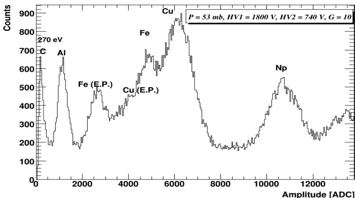
**Figure 3.** Peaks observed from the  $^{241}\text{Am}$  radioactive source through aluminium and polypropylene foil. On the left the Carbon (270 eV) peak is shown, followed by the Aluminium peak (1.45 keV), the escape peak (E.P.) of Iron in Argon (3.3 keV), the escape peak of Copper in Argon (5 keV), the Iron peak (6.4 keV), the Copper peak (8 keV) and the Neptunium peak (13.93 keV).
