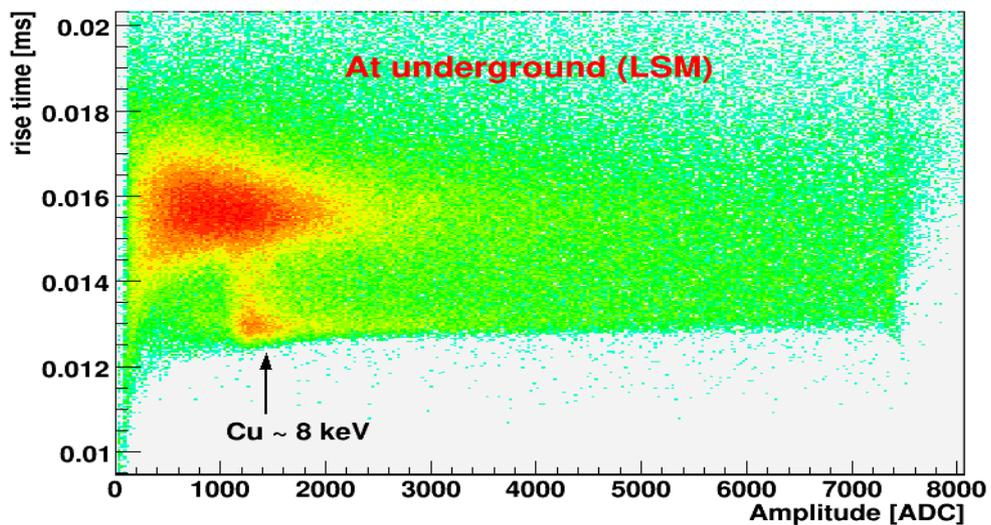
**Figure 5.** The rise time versus amplitude without source, taken at underground (P = 57 mb, HV1 = 1750 V, HV2 = 713 V at LSM).
