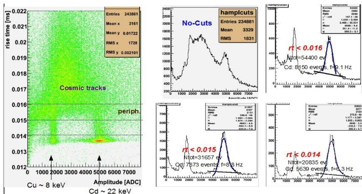
**Figure 2.** The rise time (*rt*) versus the amplitude (in ADC) of the <sup>109</sup>Cd source and the energy spectrum with the energy lines of 8 and 22 keV respectively, for various cuts in rise time (*P* = 107 mb, *HV1* = 2520 V, *HV2* = 1036 V, *G* = 20).
