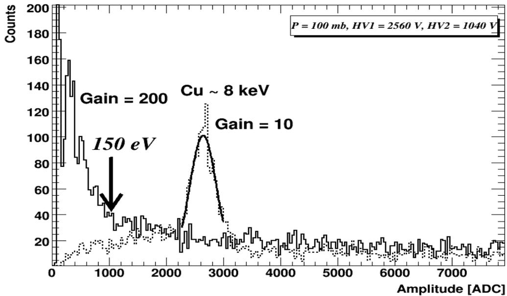
**Figure 4.** The energy spectrum at Gain = 10 with the Copper peak of 8 keV (dashed line) and at Gain = 200 where the single electron peak at ~ 50 eV is clearly visible (full line).
