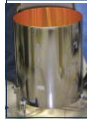
A 50-cm diameter electroformed Ni-alloy prototype for Constellation-X, produced at MSFC
