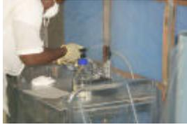
Hand spraying of epoxy onto substrate
