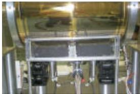
Attachment of substrates to mandrel under vacuum
