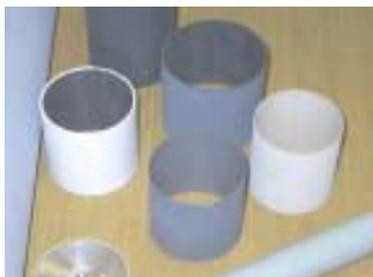
**Fig. 2.** The test shells produced by plasma spraying (light ceramics replication)
