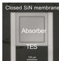
Single pixel microcalorimeter
