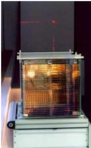
**Fig. 1.** The optical tests (with the focal image) of the prototype of a segmented mirror assembly based on gold-coated 30 cm x 30 cm glass foils
