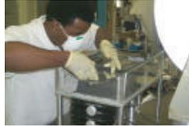
Insertion of sprayed substrate into vacuum attachment housing
