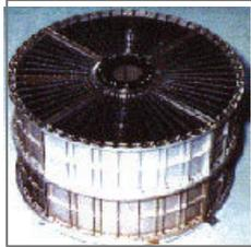
An Astro-E flight mirror, an example of a multiply nested, light weight, segmented mirror developed at GSFC
