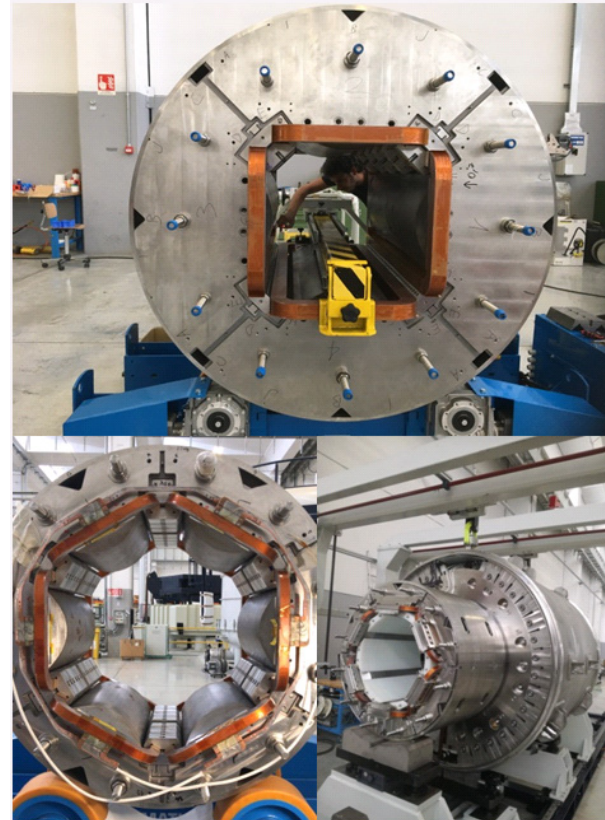
Figure 3: Quadrupole magnet assembly (top). The coil position is being checked with a laser tracker. Sextupole magnet assembly (bottom left) and magnet column on an alignment bench (bottom right).
