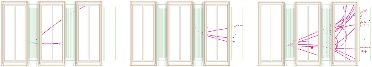
FIG. 3: ND280 tracker event displays for various topologies, from left: CC- $0\pi$ , CC- $1\pi$ , CC-Other.
