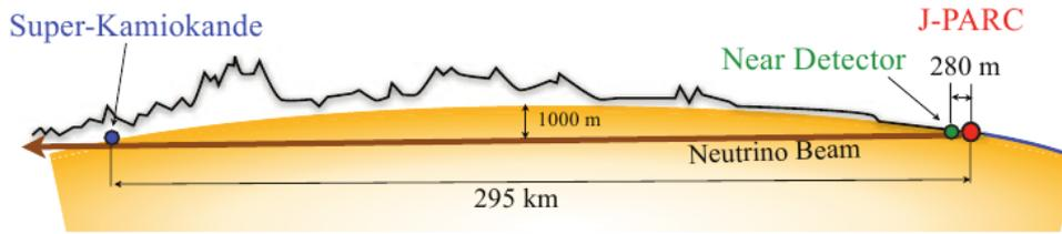
FIG. 1: Neutrinos are produced at J-PARC in Tokai, from which they travel 295km through the Earth before reaching the Super-Kamiokande detector in Kamioka. The near detector site located at J-PARC is used to monitor beam flux as well as measure neutrino interactions.
