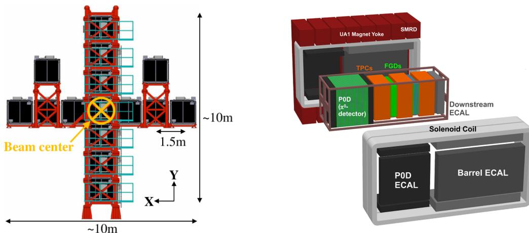
FIG. 2: Schematics of the on-axis (INGRID, left) and off-axis (ND280, right) detectors.
