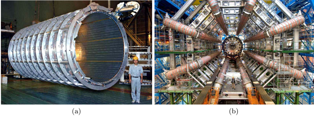
Figure 3.14: Pictures of the ATLAS magnets. (a) The solenoid magnet provides the magnetic field required for the inner detector momentum measurements and (b) the picture of the barrel toroid magnet installed in the ATLAS cavern, consisting of 8 coils in the barrel and coils regions.
