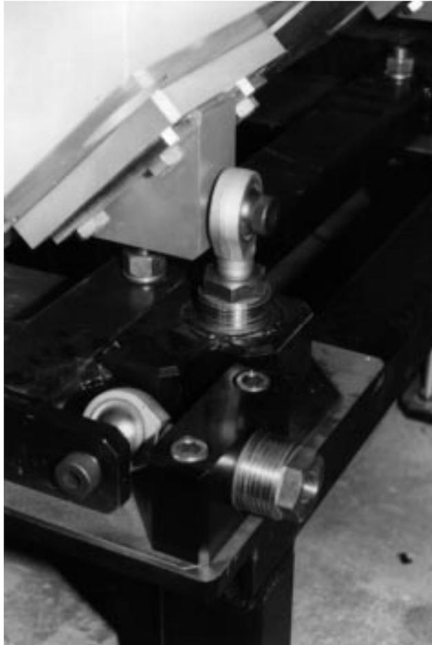
Fig. 18. Lateral adjustment layout.
