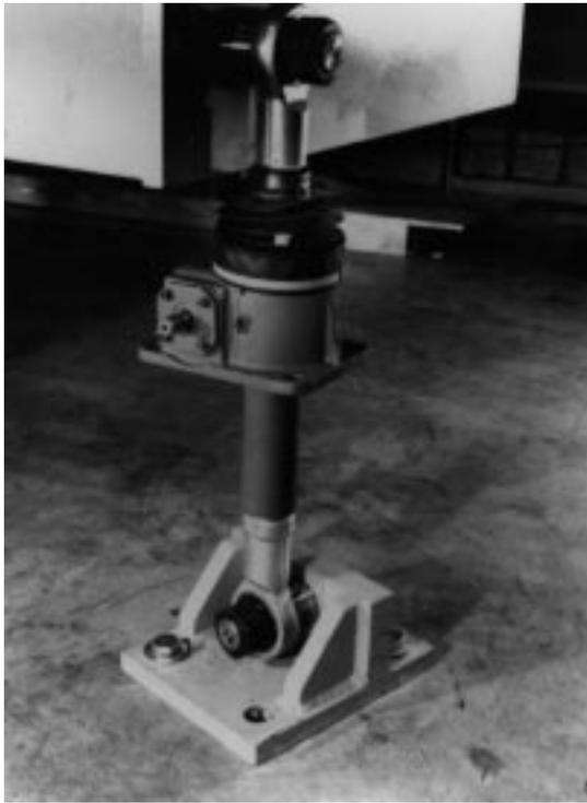
Fig. 10. ALS 5-ton machine screw jack strut.
