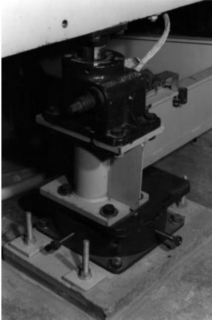
Fig. 6. Machine screw jack support.
