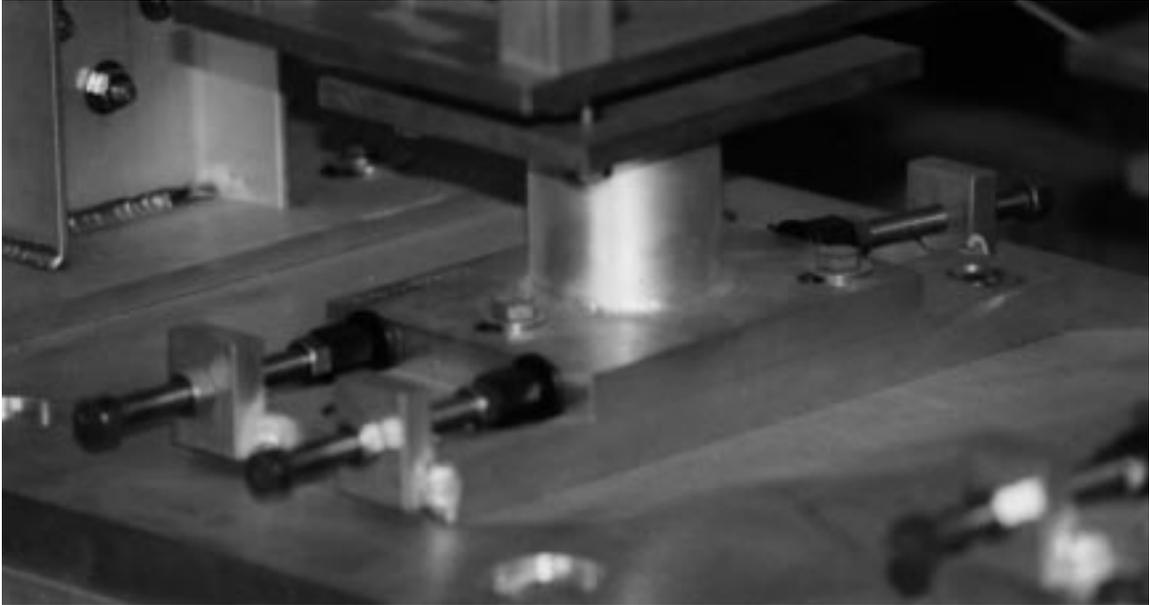
Fig. 5. Push-push screw arrangement.
