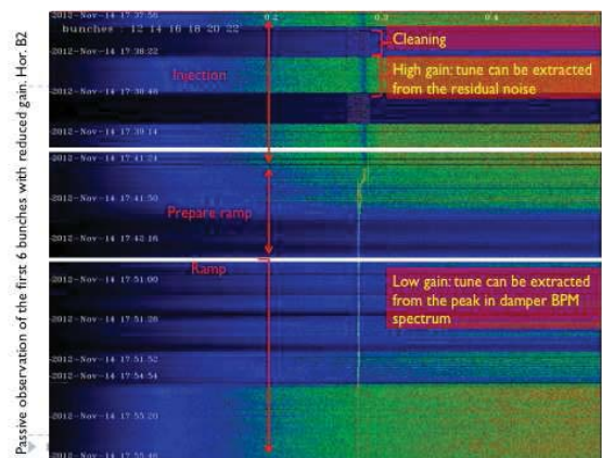
Figure 8: Result of tune observation with ADT on six witness bunches (horizontal plane, beam 2).
