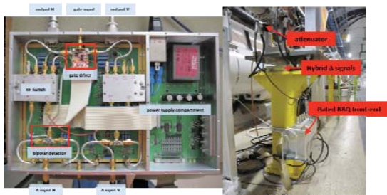
Figure 8: Picture of the Gated BBQ and its implementation in LHC Tunnel
