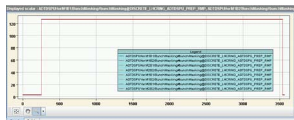
Figure 3: Gain modulation function within the turn.
