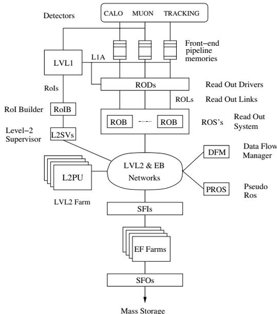
Figure 1: *The ATLAS Trigger/DAQ system.*
