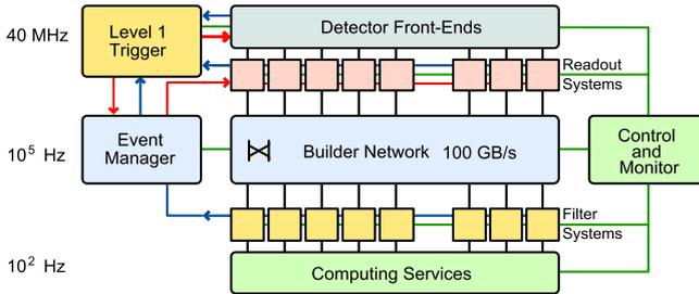
Figure 2: *Schema of CMS Data Acquisition system.*
