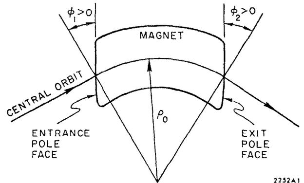
FIG. A-1--Field Boundaries for a bending magnet.
